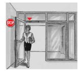
The **mechanical hold-open device** enables doors to be held without fallback at an opening angle up to approx. 120°.
